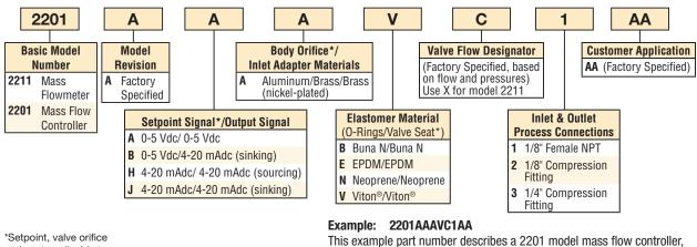
\*Setpoint, valve orifice and seat applicable to Model 2201 only
